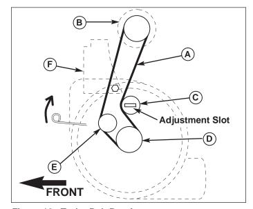
Figure 10. Turbo Belt Routing
